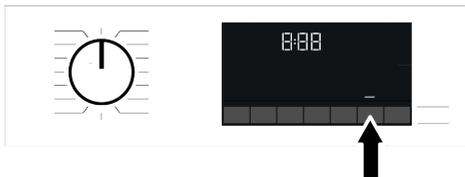
In order for the End Time function to be activated and the programme is completed at the end of the specified time, you must press Start/Pause button after adjusting the time.
