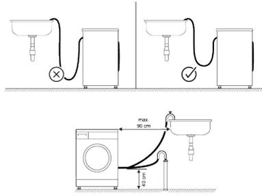
2. Connect the hose to a minimum height of 40 cm and a maximum height of 90 cm.
