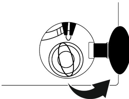
3. Pull down the loading door emergency handle with a tool and release. Then open the loading door.
