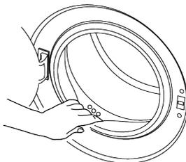
After every washing make sure that no foreign substance is left in the product. If the holes on the door gasket shown in the figure is blocked, open the holes using a toothpick.
