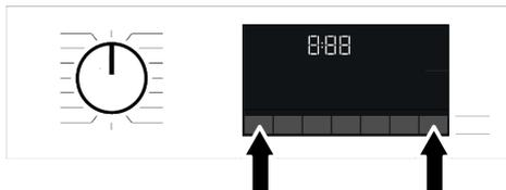
3. When the appliance is in HomeWhiz setup mode, you will see an animation on the display and the bluetooth icon will flash until your machine gets paired with smart device. Only programme knob will be active in this mode. Other buttons will be inactive.
