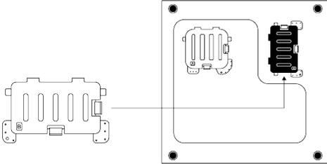
Rest the tabs of Cover B against the lower panel. Complete the assembly by rotating the cover.
