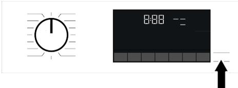
If the water level in the machine is not suitable when you press Start/Pause button, the door lock cannot be deactivated and the door lock icon on the display remains on.
