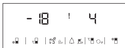
Indicator panel while the high temperature alarm is off
