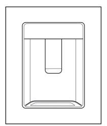
Please note, how much water flows from the dispenser depends on how far you depress the lever. As the level of water in your cup / glass rises, gently reduce the amount of pressure on the lever to avoid overflow. If you slightly press the arm, the water will drip; this is guite normal and not a failure.
