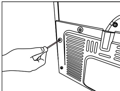
1. To install the wedges, remove the screws on the product and use the screws supplied together with the wedges.
