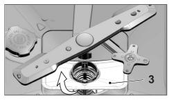
Press the two pawls on the coarse filter inwards and separate the coarse filter from the assembly.
