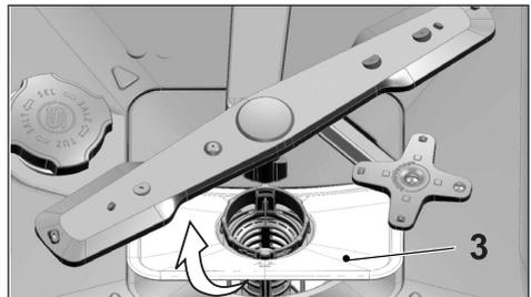
3. Press the two pawls on the coarse filter inwards and separate the coarse filter from the assembly.
