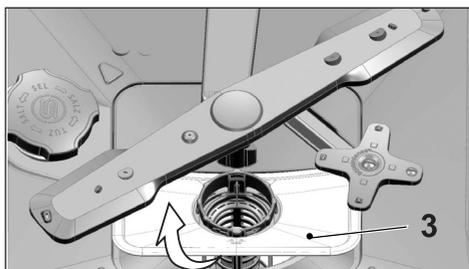
3. Press the two pawls on the coarse filter inwards and separate the coarse filter from the assembly.
