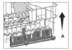
Make sure that both sides of the loaded basket height adjustment mechanism are at the same level (down or up).
