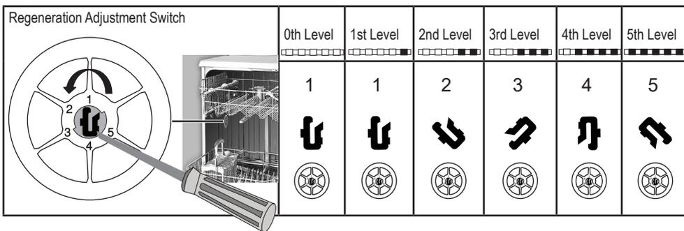
If the hardness level of the supply water is above 90 °dF or if you are using well water, then it is recommended to use water purification devices and special filters. If the hardness level of the supply water is below 13°dF, there is no need to use salt in your dishwasher. If this is the case, “No Salt Warning Indicator” (if any) illuminates continuously on the panel of your machine.
