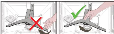
**i** Do not try to rotate the impeller by holding its ends. Trying to rotate the end sections may cause the gear system within the impeller to break.
