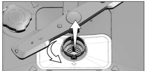
2. Pull out the metal/plastic filter (3) from the seating.
