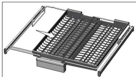
When the central tray is in the lower position, you can load long/high items such as coffee cups, ladles, etc. on the tray. When the side trays lean on two side walls, the handle can be pulled to allow the central tray to rise and the system to be locked.
