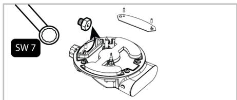
**i** On some hob burners, the injector is covered with a metal piece. This metal cover must be removed for injector replacement.
