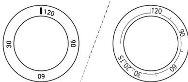
The timer has no effect on the oven functions. It is used for warning purposes. For example, you can use the alarm clock when you want to turn the food in the oven at a certain time. As soon as the time you set is up, the timer emits an audible signal.
