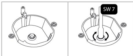
5. If your product has a wok combustor with a side-entry injector, remove the injector with a number 7 spanner.
