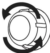
3. If your oven lamp is type (A) shown in the figure below, rotate the oven lamp as shown in the figure and replace it
