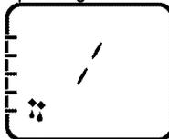
The oven is not heated. Only the fan (in the rear wall) is in operation. Suitable for thawing frozen granular food slowly at room temperature and cooling down the cooked food.
