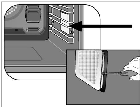
3. Lift the lamp's protective glass cover with a screwdriver. Remove the screw first, if there is a screw on the square lamp in your product.
