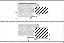
When installing the hob onto a cabinet, a shelf must be installed in order to separate the cabinet from the hob as illustrated in the above figure. This is not required when installing onto a built-under oven.
