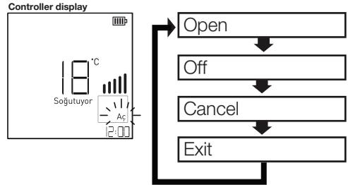
2. Set the clock using the "∧ ∨" buttons. (Each time you press the button it will change in units of 10 min.) If the button is pressed and held down for 3 seconds, the 10 minute transitions will be run faster.)
