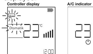
3. Press the "
