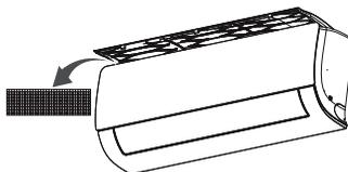
4. Remove dust and dirt from the filter with a vacuum cleaner or air. If it is contaminated, then wash with water.
