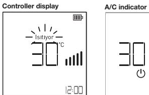
3. Press the "❄️" buttons until you reach the desired temperature. Each time you press the button, the set room temperature will increase or decrease by 1° C.
