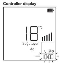
3. Press the "Onay" button (✔️) to finish setting the clock. When the setting is complete, the "Aç" symbol will appear on the remote control and the current time will be displayed.
