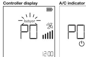
4. To cancel the rapid heating function, simply press one of these buttons: "Fast", "Silent", "⚡ / ⚡", "❄️", "Energy Control", "Cool", "Heat" and "Mode". With the quick rapid function cancelled, the A/C will continue to operate at the highest fan speed (except silent, ⚡ / ⚡). To change the speed, see "Fan speed adjustment"
