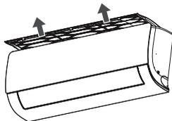
4. Clean the air filters with vacuum or warm water. If the air filter is too dirty, wash it in warm detergent water.
