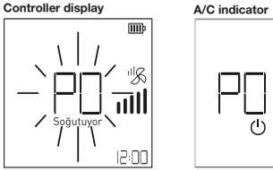
4. To cancel the rapid cooling function, simply press one of these buttons: "Fast", "Silent", "Energy Control", "⚡ / ⚡", "❄️", "Cool", "Heat" and "Mode". With the quick rapid function cancelled, the A/C will continue to operate at the highest fan speed (except silent and power-saving, ⚡ / ⚡). To change the speed, see "Fan speed adjustment"
