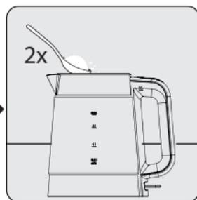
Pour 1 cup of white vinegar or 2 tablespoons of lemon salt into the boiling water. After letting it sit for a few hours, drain the water and rinse it thoroughly. Operate the device once again with only water.
