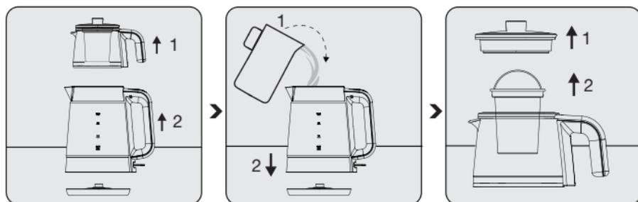
Remove the kettle (5) from the base unit (7) after lifting the teapot (2).
