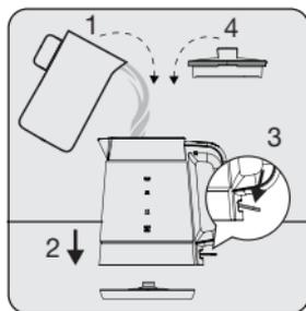
Fill the kettle (5) to the max. line and place it on the base unit (7). Push the on / off switch (6) down slightly to the ON (I) position.
