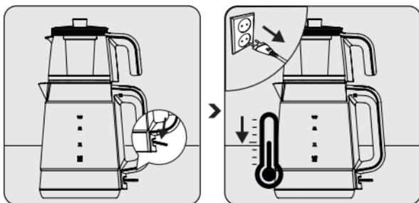
When use is finished, push the on / off switch (6) down slightly to the OFF position (0).
