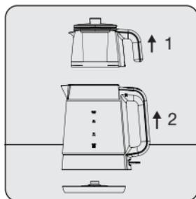
Remove the kettle (5) from the base unit (7) after lifting the teapot (2).
