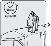
If you do not move the appliance for 8 minutes while in vertical position, it would shut-down automatically.
