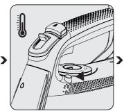
Set the temperature adjustment button (6) to the "MAX" position and wait until the thermostat light (10) turns off.
