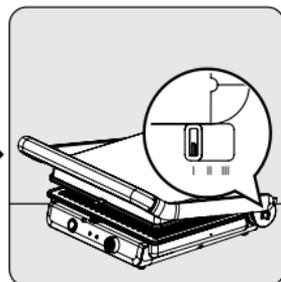
Set the level adjustment slider (2) to the desired level ( I - II - III ) and close the top handle (9) downwards.
