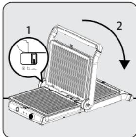
Move the top cover of the appliance to the “
