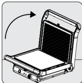
Open the top cover of the appliance upwards by holding the handle (9).
