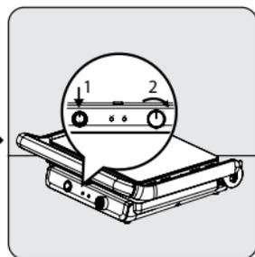
To start the appliance, turn the On/Off switch (8) to the "I" position. Set the thermostat knob (6) to the position you want to cook.
