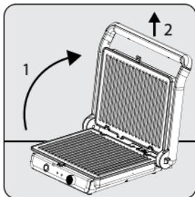
Open the top cover of the device by holding the handle (8). Then pull it upwards.
