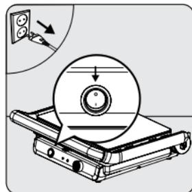
To turn off the appliance, turn the On/Off switch (8) to the "0" position and unplug it.
