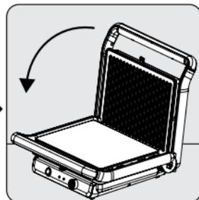
Close the top cover of the appliance downwards by holding the handle (9).
