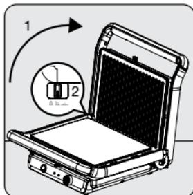
Lift the top cover of the appliance slightly and move the locking slide (1) to the half-open "□" position. Open the top cover of the appliance upwards by holding the handle (9).
