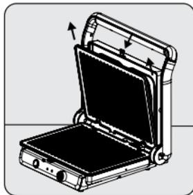
Press the plate locking latches on the front of the upper and lower cooking plates (10) and lift up slightly to remove the plates.
