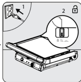
Push the locking slide (1) to the half-open "I" position.
