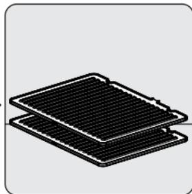
To reinsert the cooking plates (10), insert the cooking plates into the slots on the inside back of the appliance and snap them into place.
