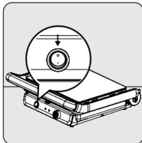
To turn off the appliance, turn the On/Off switch (8) to the "0" position.
