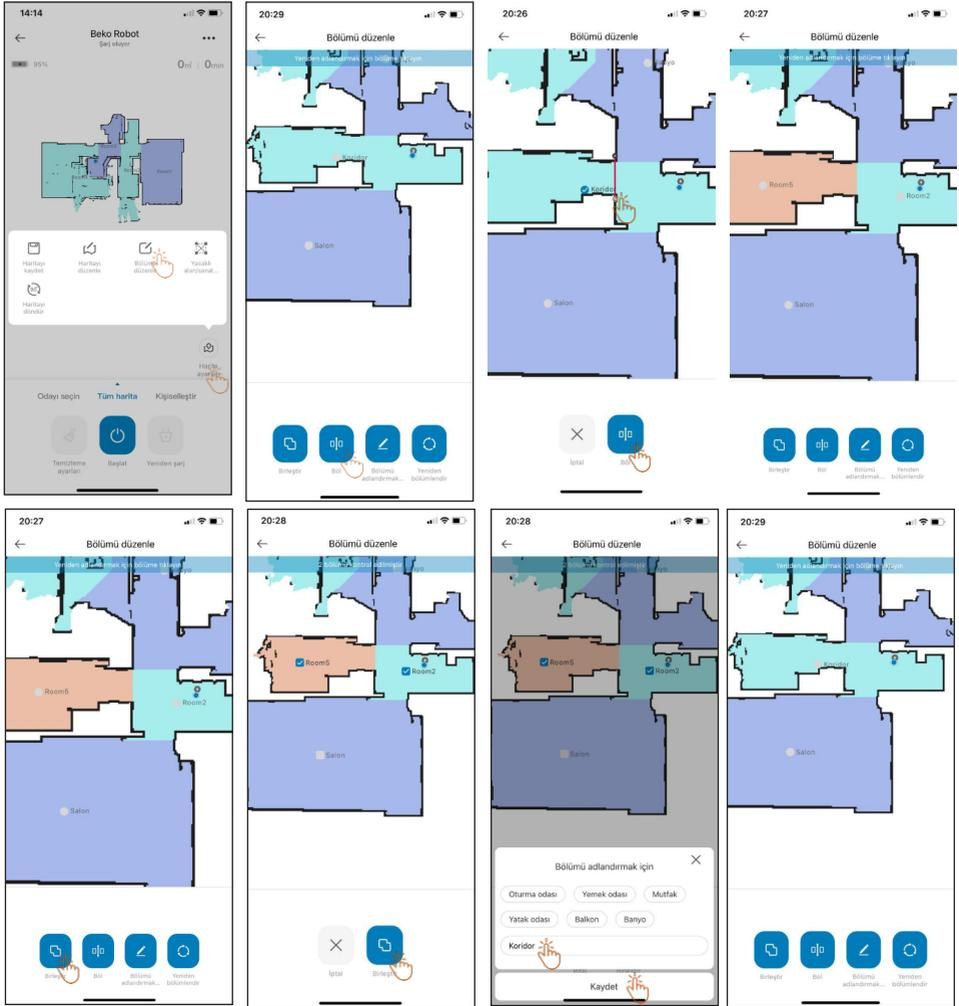
17. You can permanently add **"Restricted Areas"** and/or **"Virtual Walls"** in areas where you do not want the robot to go. (For ex.: If you have furniture that is lower than the height of the robot, it is recommended to define a restricted area to prevent the device from getting stuck under the furniture).
