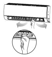
One-touch soft air ( ) When the " " button is pressed, it easily adjusts the air flow at two different angles to deflect the directly incoming wind.
