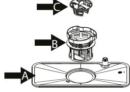
The filter system consists of a coarse filter, a flat (Main filter) and a micro filter (fine filter).
