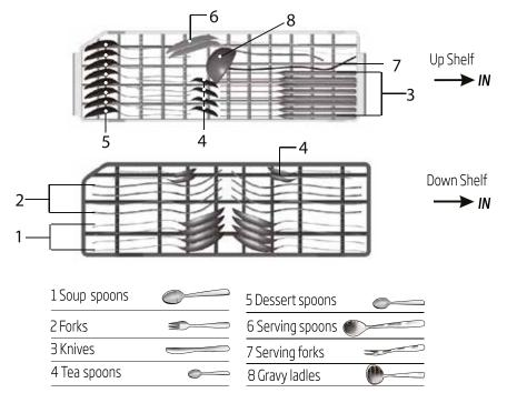
Information for comparability tests in accordance with EN 50242 Capacity: 8 place settings
