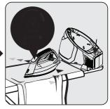
Auto shut off "U" indicator will turn off after you move the iron or push any button. LED display (1) will blink until the iron is ready again.
