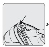
Place the iron on the dock (10) and push on the carrying lock (15) to lock the iron.
