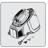
Pull and release the power cord. Cable will be wrapped into the wrapping slot (17).
