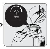
To exit turbo steam mode, push the level adjustment button (3). - Turbo steam symbol "命命" will disappear from the display.
