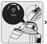
Set the fabric-appropriate temperature and steam using the level adjustment button (3). (See 3.6)
