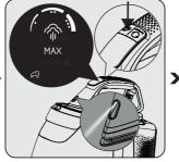
Push the automatic steam button (2) to activate automatic steam function.
