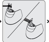
Remove the water tank (11) by holding it from the tank detaching handle (13) and pulling.
