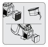
To empty the calc box (8), open the lid (7) and empty. Then, make sure the calc box (8) is properly seated.
