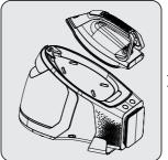
The lock will be unlocked and you will be able to lift the iron from the dock.
