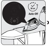
Iron will automatically turn off if it does not move horizontally for 30 seconds or any buttons are pressed.
