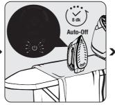
Iron will automatically turn off if it does not move vertically for 8 minutes or any buttons are pressed.
