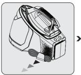
Pull the steam cable clip (9) and place the cable.
