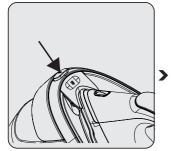
To detach the iron from the dock, push on the carrying lock unlock button (14).
