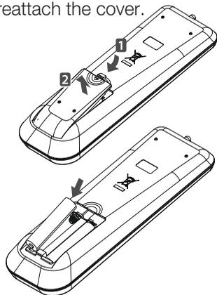
**i** If the display of the remote control disappears, reinstall the batteries.
