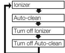
2. To switch off the Ionfresh air purge function, press the Ion/Cleaning button until the "Ionizer" symbol in the control display goes out.
