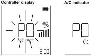
4. To cancel the rapid cooling function, simply press one of these buttons: "Fast", "Silent", "Energy Control", "🌀/🌀", "⬆️", "Cool", "Heat" and "Mode". With the quick rapid function cancelled, the A/C will continue to operate at the highest fan speed (except silent and power-saving, 🌀/🌀). To change the speed, see "Fan speed adjustment"
