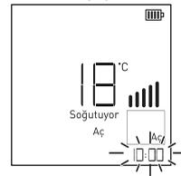
3. Press the "Onay" button (✔️) to finish setting the clock. When the setting is complete, the "Aç" symbol will appear on the remote control and the current time will be displayed.
