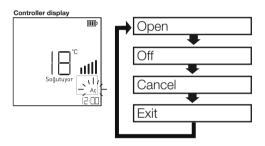
Set the clock using the "∧∨" buttons. (Each time you press the button it will change in units of 10 min.) If the button is pressed and held down for 3 seconds, the 10 minute transitions will be run faster.)
