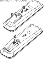
(1) If the display of the remote control disappears, reinstall the batteries.
