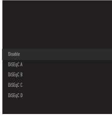
Select »DiSEqC A«, »DiSEqC B«, »DiSEqC C« or »DiSEqC D« to select the satellite corresponding to the respective DiSEqC positions in the satellite system.
