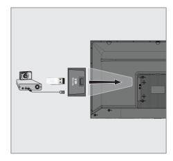
Connect the USB interface of the television and the corresponding socket on the data device (external hard drive, digital camera, card reader or MP3 player) using a USB cable;
