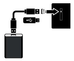
Connect the »USB« interface of the television and the corresponding socket on the data device (external hard disk, digital camera, card reader or MP3 player) using a USB cable.
