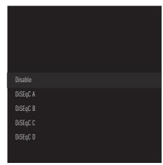
Select »DiSEqC A«, »DiSEqC B«, »DiSEqC C« or »DiSEqC D« to select the satellite corresponding to the respective DiSEqC positions in the satellite system.
