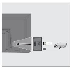
Plug the external hard disk to the USB USB interface of the television.
