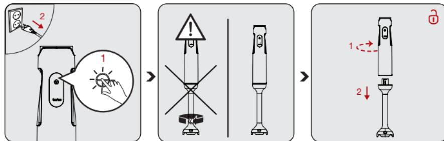
When process is complete, release the power button (2). Unplug the appliance.
