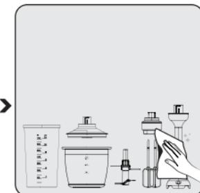
Unplug the appliance before cleaning. Make sure that all appliance components has stopped completely. Wipe the motor unit (4) of the appliance with a damp cloth.
