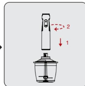
Place the motor unit (4) onto the chopping cover (6).
