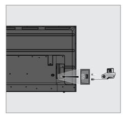
Connect the **USB (HDD)** interface of the television and the corresponding socket on the data device (external hard drive, digital camera, card reader or MP3 player) using a USB cable.
