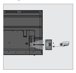
Plug the external hard disk to the USB (HDD) USB interface of the television.
