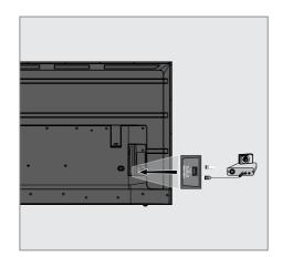
Connect the USB (HDD) interface of the television and the corresponding socket on the data device (external hard drive, digital camera, card reader or MP3 player) using a USB cable.
