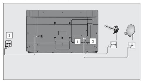
To receive digital satellite channels (DVB-S), connect the satellite antenna cable to the **»SATELLITE**« antenna socket on the television set;
